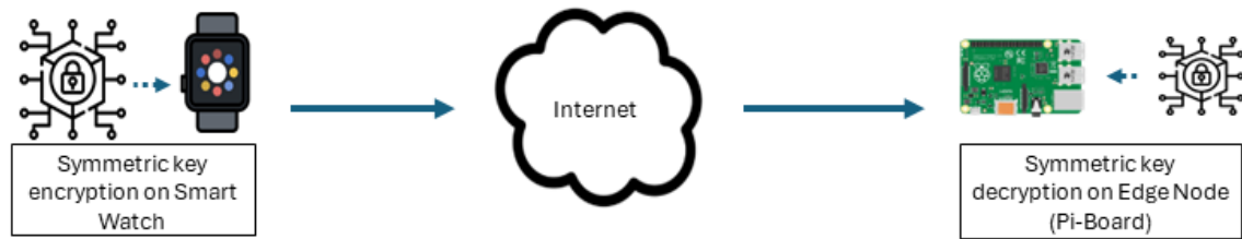
Figure 23: Encryption on Sensing Devices and Decryption on Fog-node
